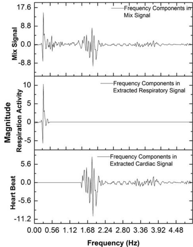
**Figure 4** Plots processed in frequency analysis method representing the mixed signals in frequency domain for extraction of respiratory and cardiac activity.
