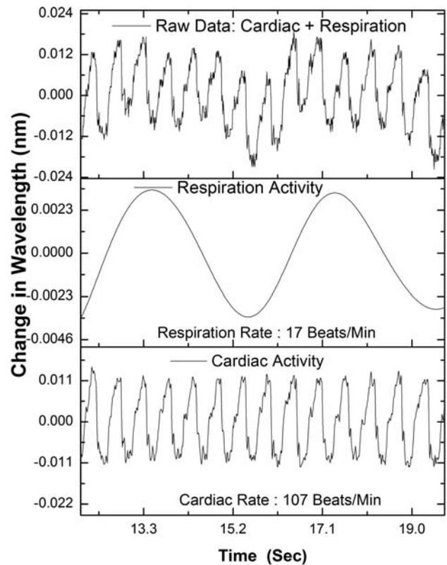
**Figure 6** Expanded view of two respiratory cycles from Figure 5 which illustrates the quality of single recording and superiority of extracted morphology of each beat.
