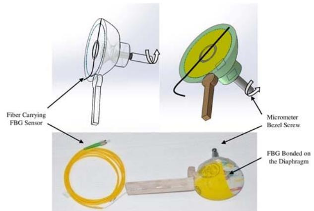
**Figure 1** Design schematics and pictorial representation of FBGHBD.
