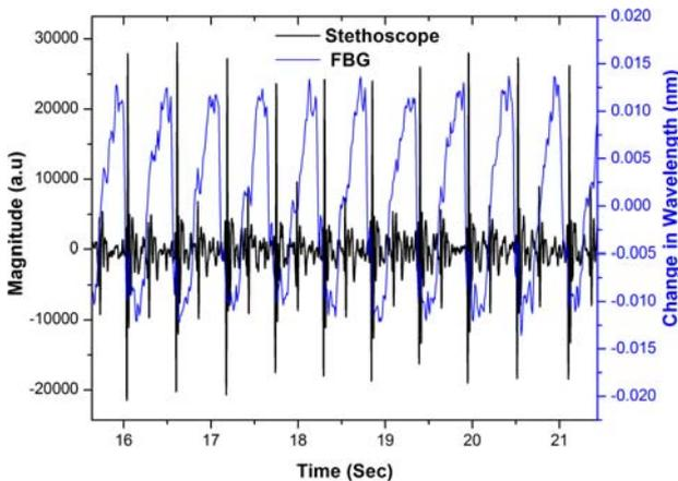
**Figure 8** Expanded view of FBGHBD and stethoscope signal for 10 heart beat cycle.
