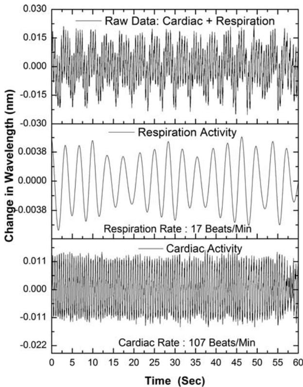
**Figure 5** Plots processed in frequency analysis method representing the mixed signals in time domain for extraction of respiratory and cardiac activity.
