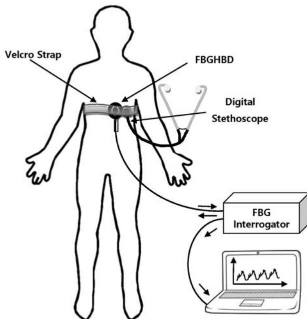
**Figure 2** Schematic representation of the experimental setup.
