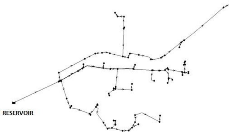
Figure 2: Schematic and water flow direction in Mandya water distribution network
