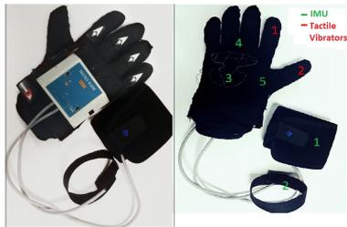
Fig. 4: Positioning of IMUs and actuators in the tactile glove
