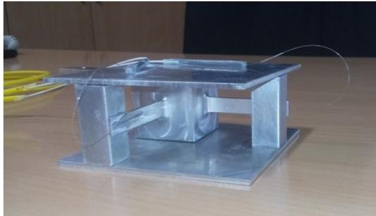
Figure 2. Pictorial representation of FBG Accelerometer device.
