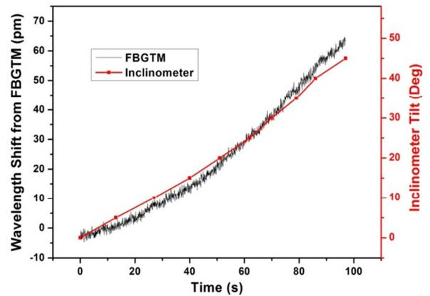
Figure 4. Comparison of FBGTM response with inclinometer response during calibration.
