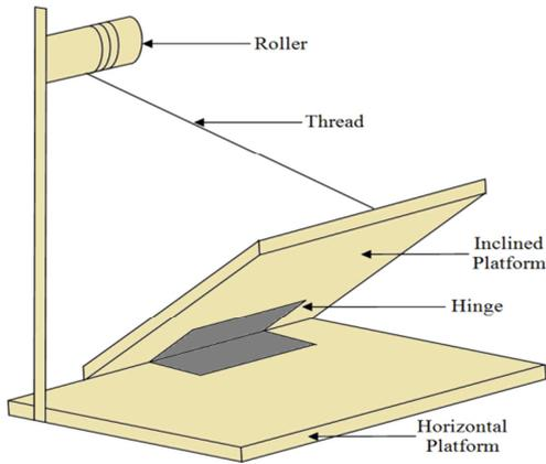
Figure 2. Schematic of tilt platform used in the experiment.
