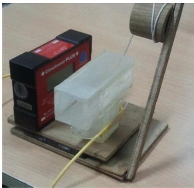
Figure 3. Experimental setup with FBGTM and inclinometer.
