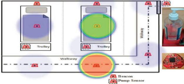
Figure 1: Tracking and monitoring infrastructure of the *CleanHands* system. Heat map of the movement of people in the mockup ICU.
