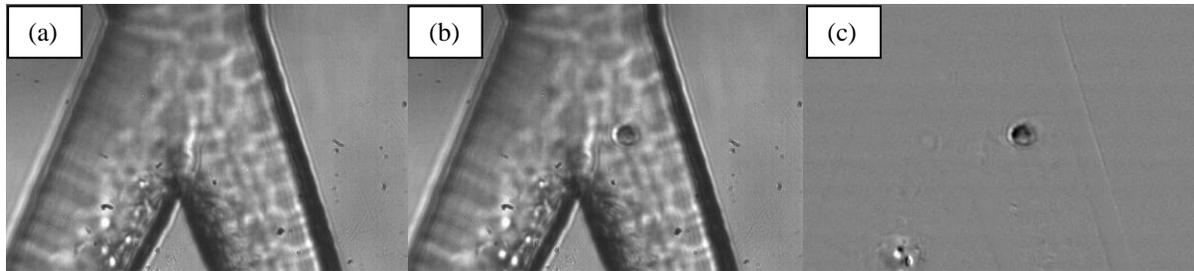
Figure 4 : (a) Background image not containing any cells. (b) Frame containing a cell before background subtraction. (c) Frame containing cell after background subtraction.
