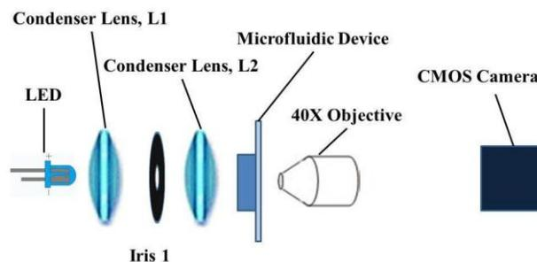
Figure 3: Experimental setup used for characterization of glass microfluidic channels
