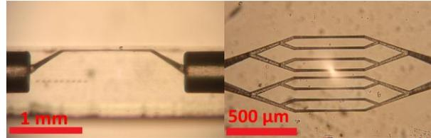
Figure 2: Device after etching. (a) Side view of the device showing the channel moving up to the surface for imaging. (b) Top view showing the individual channels.
