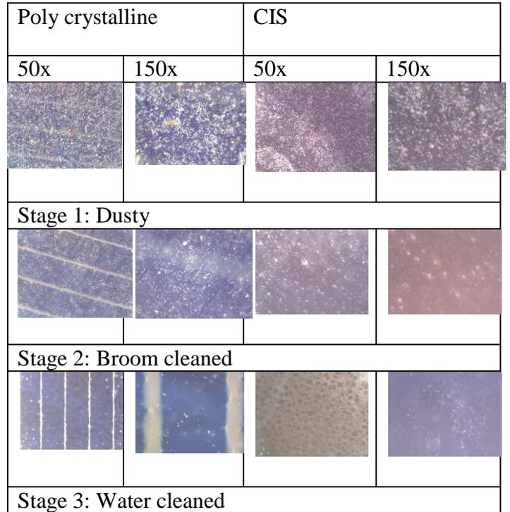
Fig 1. Optical images of the PV panel surface at various cleaning stages (Magnification of 50x and 150x using a 19" monitor)
