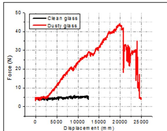
**Fig 4.** Micro-indentation force measurement on a clean vs dusty surface
