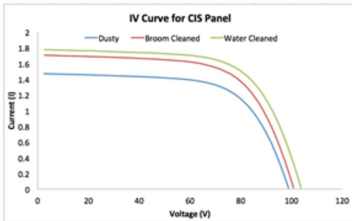
Fig 5. IV characteristics for Poly-Si and CIS panels at various stages of cleaning
