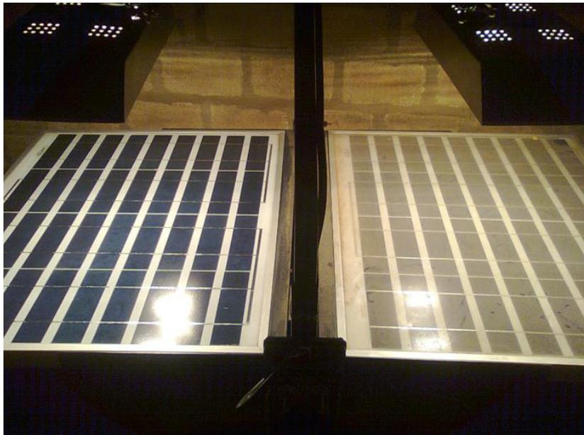
Fig. 1. Indoor solar simulator setup.
