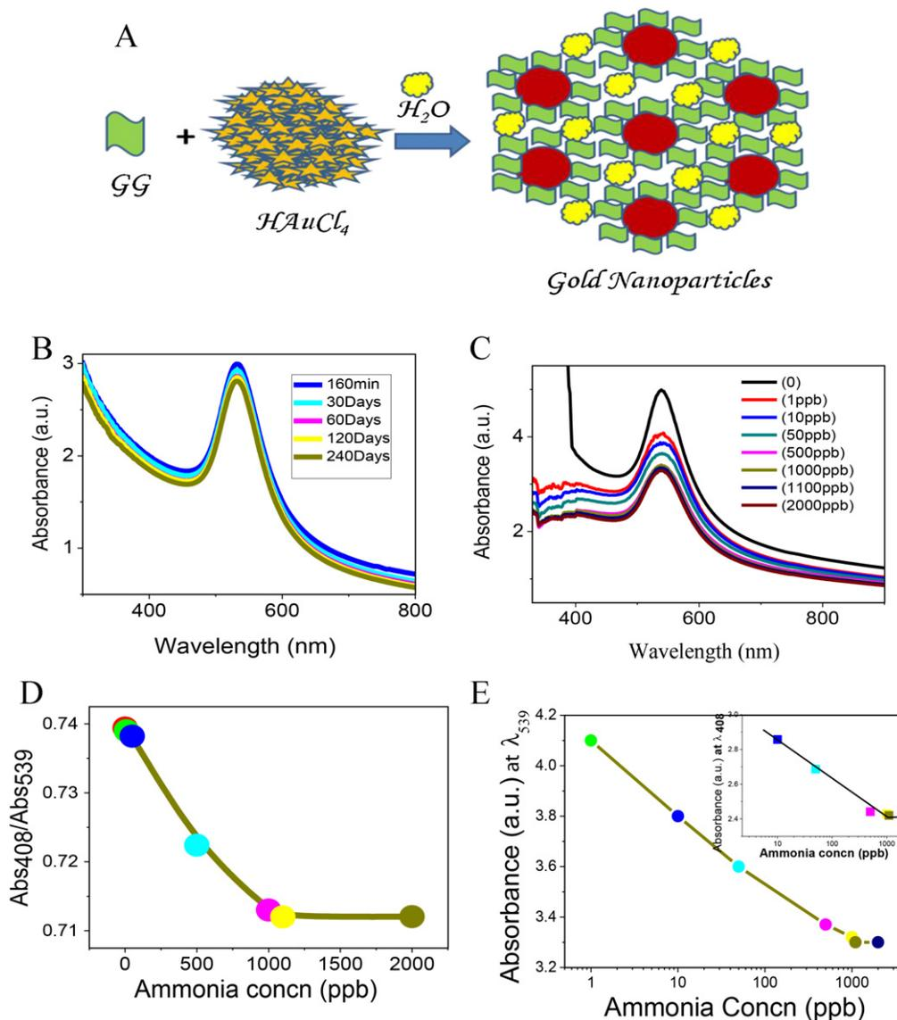
**Fig. 3.** (A) Mechanism for stabilization of NPs. (B) Stability of AuNPs. (C) Plot of change in spectral absorbance as a function of ammonia concentration. (D) Ratio of absorbance of wavelength ( $\lambda_{408}/\lambda_{539}$ ) as a function of ammonia concentration. (E) Variation in absorbance at  $\lambda_{539}$  and  $\lambda_{408}$  (inset) as a function of ammonia concentration.
