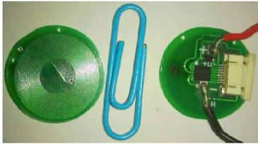
Fig. 4. Coil with charger circuit
