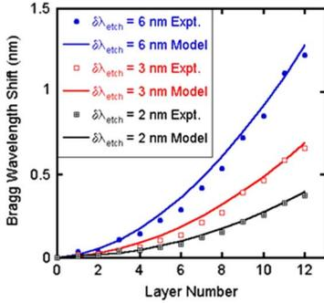
Fig. 7. Measurement of LbL assembly of PAH/PAA system at a deposition pH of 5.5 using 3 EFBG sensors with different fiber diameters, and consequently different surface adsorption sensitivities. The data can be fitted nicely using the adsorption model given by (3a) by varying only the fiber diameter as a parameter in the numerical model.
