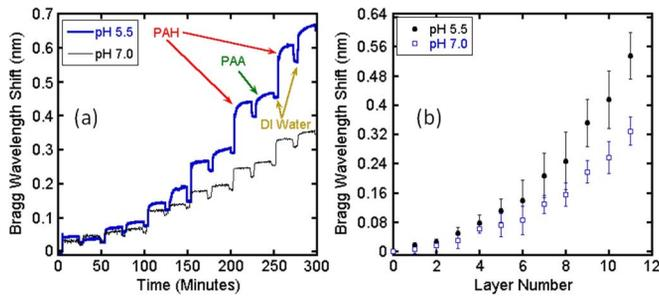
Fig. 5. LbL assembly of weak polyelectrolytes (PAH/PAA) measured in real-time with EFBG sensors. Fig. 5(a) is the real-time data and Fig. 5(b) shows the layer buildup with odd layer numbers corresponding to PAH and even layer numbers corresponding to PAA.
