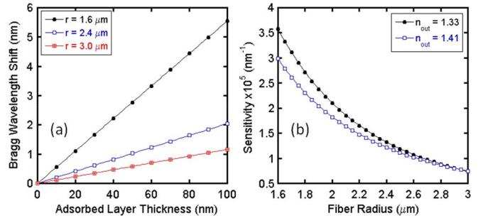
Fig. 4. a) Bragg wavelength shift due to surface adsorption calculated using the FEM model, showing a good linear behavior. Fig. 4 b) shows that sensitivity of the EFBG sensor increases faster than linearly with decreasing fiber diameter.
