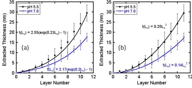
Fig. 6. Layer growth behavior of PAH/PAA LbL assembly modeled using an exponential, 6(a), and a quadratic, 6(b), growth equation as a function of layer number.
