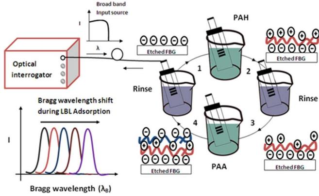
Fig. 1. Schematic of real-time monitoring of LbL assembly of polyelectrolytes using EFBG sensors.
