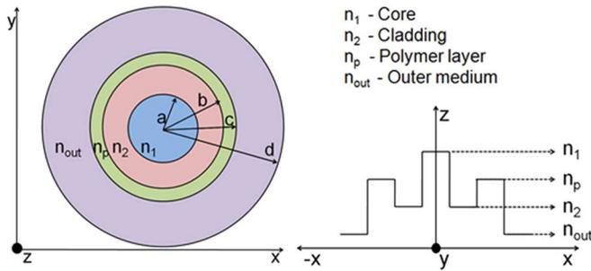
Fig. 2. Cross-sectional view of the FEM model constructed using COMSOL package to calculate the effective index change due to surface adsorption.
