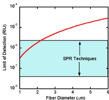
Fig. 8. Comparison of LoD of FBGs with those reported in literature [28] for SPR. FBGs attain competitive performance when etched below 2 microns.
