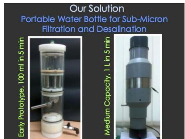
Test results of the filtration effect and prototype of the portable water bottle as presented for Google Zurich
